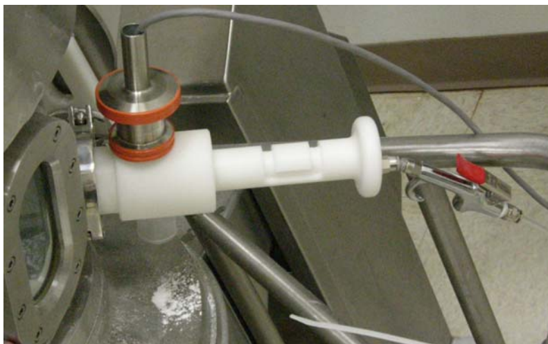
Figure 1: Sample valve with Effusivity sensor
