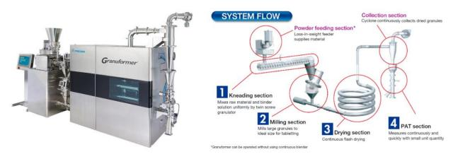
Fig. 1 Continuous Manufacturing System Granuformer® appearance and system flow chart Source: "Freund Corporation Granuformer® Catalog"
