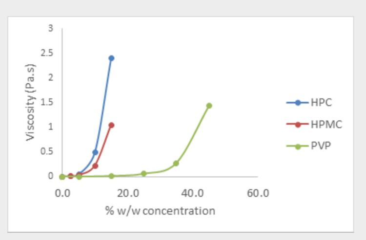
Figure 3. Viscosity of PVP, HPMC, HPC at 20 °C
